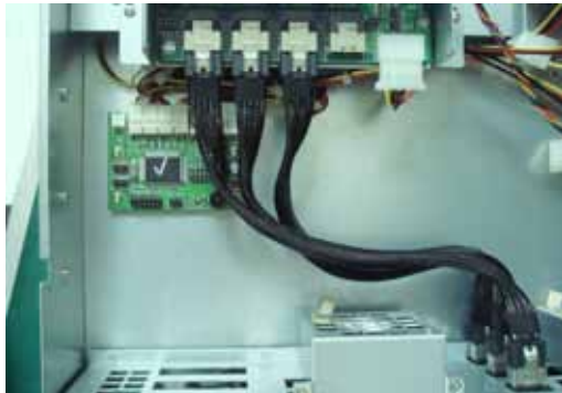
Figure 2-5, Connect ARC-8020 and backplane
